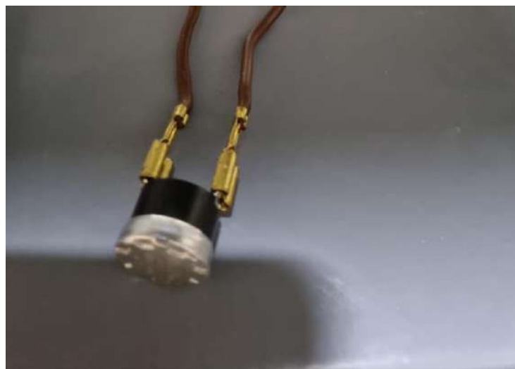
Photo 6. Thermal cut-out
